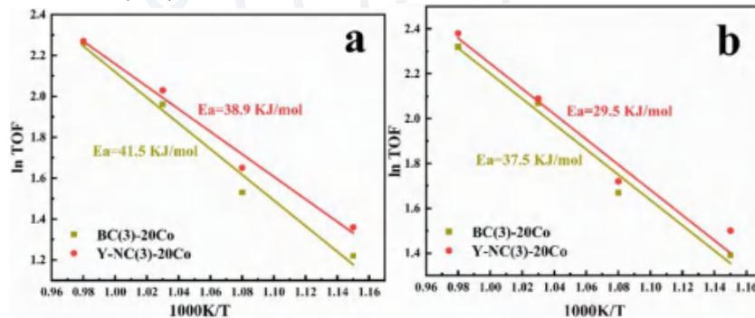
Fig 10 Arrhenius plots for the methane dry reforming over BC(3)-20Co and Y-NC(3)-20Co: (a) CH<sub>4</sub>; (b) CO<sub>2</sub>
