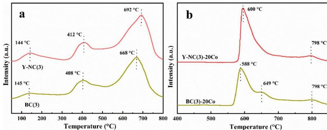
Fig 7 (a) CO<sub>2</sub>-TPD on metal-free BC(3) and Y-NC(3) and (b) CH<sub>4</sub>-TPD on BC(3)-20Co and Y-NC(3)-20Co
