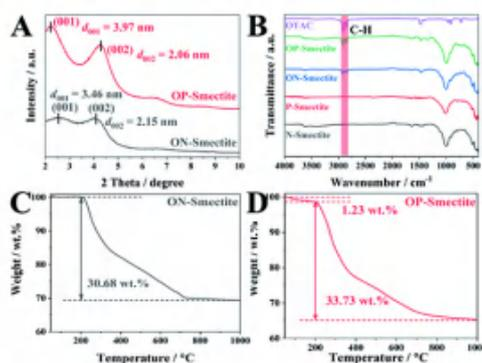
Fig. 3. Organic intercalated natural smectite (ON-smectite) and synthetic smectite (OP-smectite): (A) XRD patterns, (B) FT-IR spectra, and thermogravimetric traces (C: ON-smectite; D: OP-smectite).
