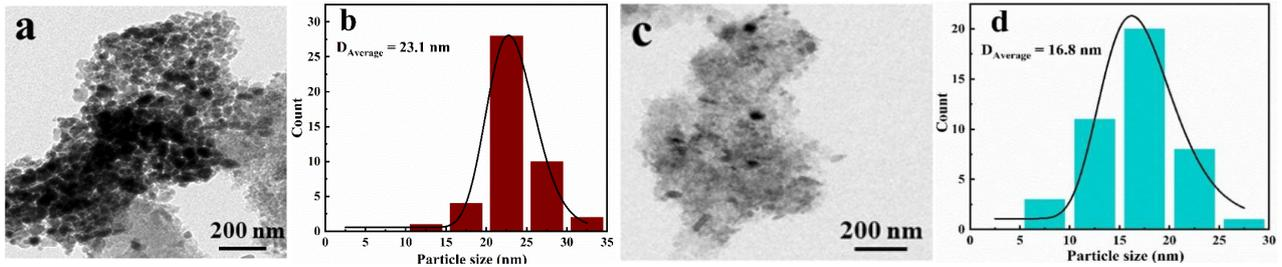
Fig 2 (a) TEM image and (b) Co particle size distribution of BC(3)-20Co; (c) TEM image and (d) Co particle size distribution of Y-NC(3)-20Co
