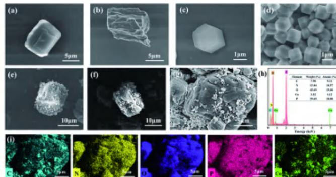
Figure 2. SEM images of APP (a), A@P (b), and ZIF-67 (c-d); SEM images (e-g), EDS (h), and elemental mapping (i) of A@P-Z.
