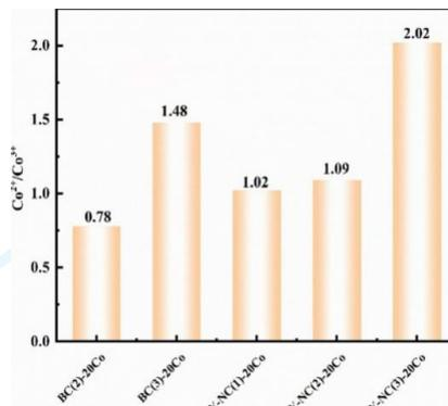
Fig 5 Co<sup>2+</sup>/Co<sup>3+</sup> value of all Co-based catalysts
