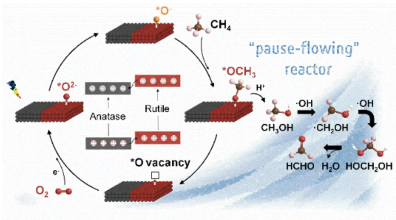
Fig 1 Selective Photooxidation of Methane to Formaldehyde via TiO<sub>2</sub> Crystal Phase Engineering in flow reactor at room temperature.
