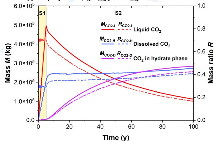
Fig. 4. Evolutions of mass  $M$  and mass ratio  $R$  of CO<sub>2</sub> component in different phases (S1: 0-5 y; S2: 5-100 y).
