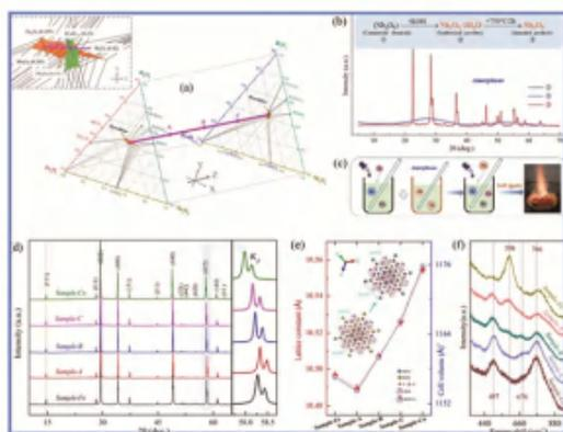
Continuous Co-level from 0 to 100% was ingeniously designed on the basis of special phase diagrams and pyrochlore-type pure samples were successfully fabricated by a modified sol-gel auto-combustion method. Significantly, two opposing structural shifts were observed with increasing the Co-level, ascribed to the competition between displacive disorders on the Bi sites and structural distortions in the octahedral network.
