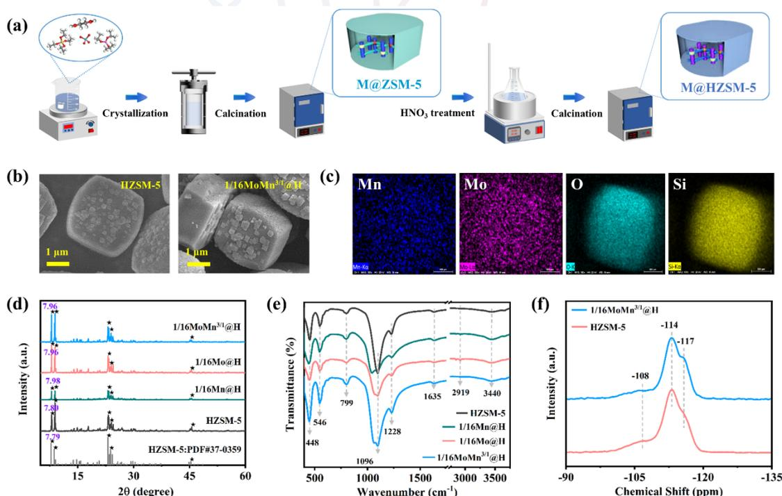
Fig 1 (a) Schematic diagram of synthesis process of catalysts; (b) SEM of HZSM-5 and 1/16MoMn<sup>3/1</sup>@H; (c) Elemental mapping of 1/16MoMn<sup>3/1</sup>@H; (d) XRD patterns of the 1/16MoMn<sup>3/1</sup>@H, 1/16Mo@H, 1/16Mn@H and HZSM-5; (e) FTIR spectra of various catalysts; (f) <sup>29</sup>Si NMR spectra of the 1/16MoMn<sup>3/1</sup>@H and pristine HZSM-5.
