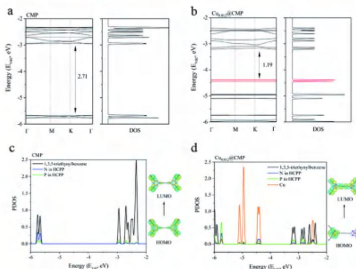
Fig. 3. Band structures and DOS of (a) CMP and (b) Cu<sub>0.012</sub>@CMP. For the purpose of comparison, the contribution of Cu SAs in the band structures was distinguished by red coloring. PDOS and HOMO-LUMO transitions of (c) CMP and (d) Cu<sub>0.012</sub>@CMP.
