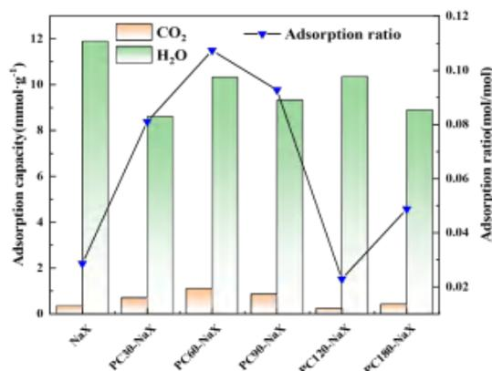
Fig 1 Adsorption capacity and separation ratio of CO<sub>2</sub> and H<sub>2</sub>O in an atmosphere of 400ppmCO<sub>2</sub> and RH40%.
