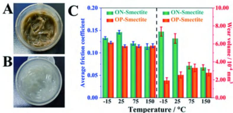
Fig. 5. Photographs of base oil and smectite grease: (A) ON-smectite grease, (B) OP-smectite grease; (C) average friction coefficient and wear volume.
