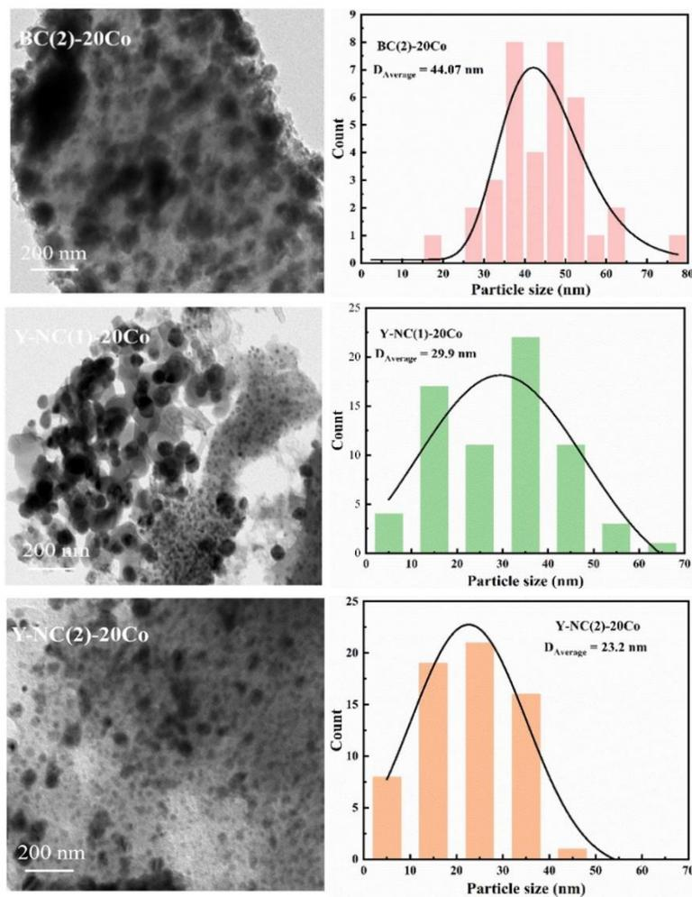
Fig 3 TEM images and particle size distribution of BC(2)-20Co, Y-NC(1)-20Co and Y-NC(2)-20Co
