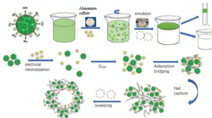
Fig 3 Microalgae harvest mechanism diagram of emulsion as buoy-bead
