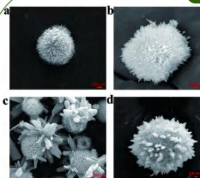
Fig. 1 SEM of (a) CuO, (b) 1ZnO@3CuO, (c) ZnO@CuO, and (d) 3ZnO@1CuO.
