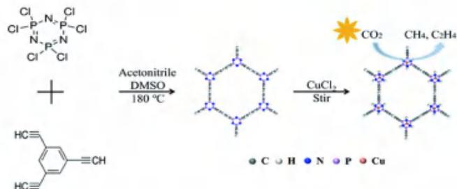
Fig 1. Synthesis and structural characterizations of Cu<sub>0.012</sub>@CMP.
