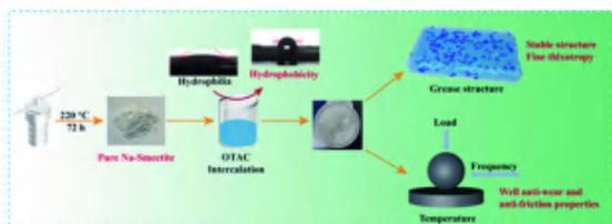
Fig. 1. Schematic diagram of synthetic smectite as a thickener.
