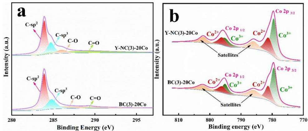
Fig 4 High resolution XPS spectra of (a) C1s and (b) Co2p in BC(3)-20Co and Y-NC(3)-20Co
