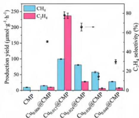
Fig 2. Photocatalytic performance and C<sub>2</sub>H<sub>4</sub> selectivity for CO<sub>2</sub> reduction of CMP with different Cu catalysts.
