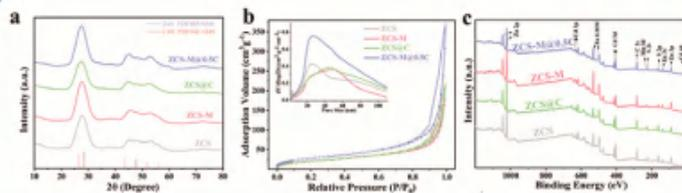
Figure 2. (a) XRD patterns, (b) N<sub>2</sub> adsorption-desorption isotherms with corresponding pore size distribution curves, and (c) XPS survey spectrum of specimens.
