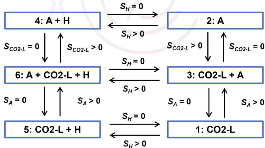
Fig. 1. Possible phase combinations in the liquid CO<sub>2</sub>-CO<sub>2</sub> hydrate system (The designations of three single phase are CO<sub>2</sub>-L – liquid CO<sub>2</sub>, A – aqueous, H – CO<sub>2</sub> hydrate).
