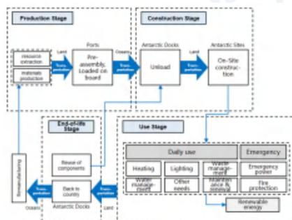
Figure 1 Calculation model of carbon emissions over the full life of an Antarctic research station
