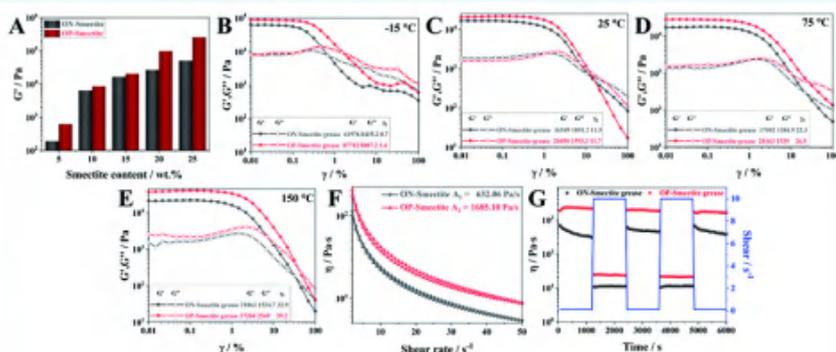
Fig. 4. Rheological properties of ON-smectite grease and OP-smectite grease: (A) storage modulus ( $G'$ ) corresponding to different thickening agent contents; (B) viscoelastic plots for smectite grease at -15 °C; (C) viscoelastic plot of smectite grease at 25 °C; (D) viscoelastic plot of smectite grease at 75 °C; (E) viscoelastic plot of smectite grease at 150 °C; (F) the thixotropic ring of smectite grease and (G) plots of apparent viscosity of smectite grease versus shear rate.
