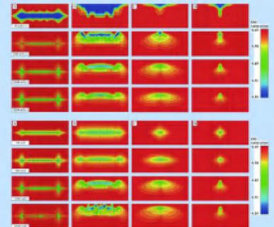
Oil saturation change diagram of influence of different reservoir permeability on production area of horizontal wells:
