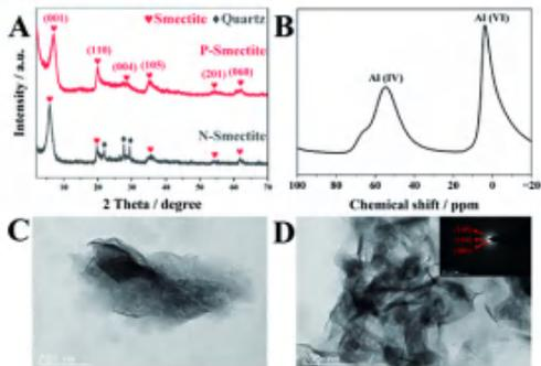
Fig. 2. (A) XRD patterns of natural smectite and synthetic smectite; (B) <sup>27</sup>Al NMR spectrum of synthetic smectite; TEM images: (C) natural smectite, (D) synthetic smectite (local electron diffraction image at upper right).
