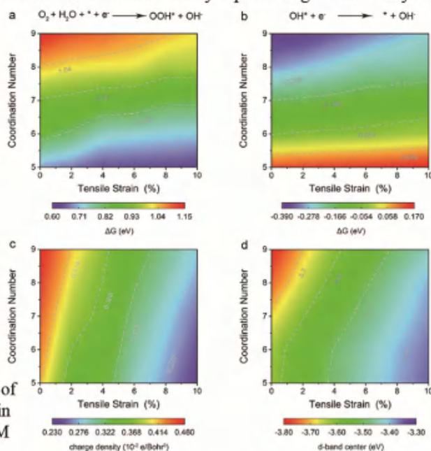
Fig 4 Theoretical calculations on the effect of CN and TS on free energy in the ORR process and the electronic structure of Ag.
