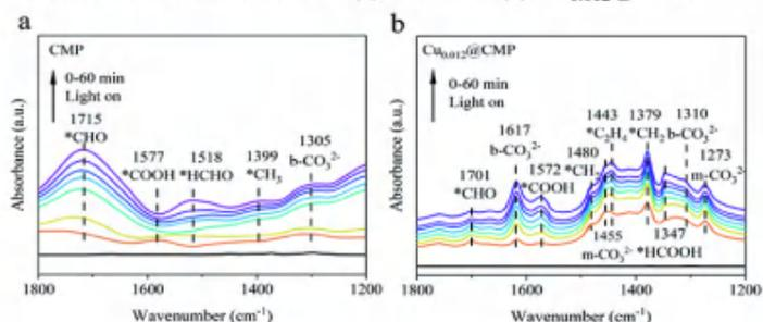
Fig 4. *In situ* DRIFTS measurement using (a) CMP and (b) Cu<sub>0.012</sub>@CMP as a catalyst under the dark and visible light irradiation, respectively.
