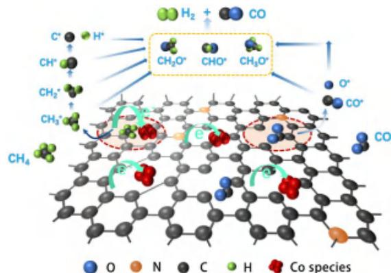
Fig 11 Possible reaction mechanism over Y-N(Z)-20Co catalyst
