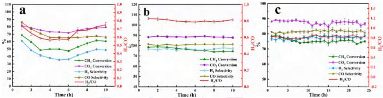
Fig 9 (a) CH<sub>4</sub> conversion, CO<sub>2</sub> conversion, H<sub>2</sub>/CO, H<sub>2</sub> Selectivity and CO Selectivity of BC(3)-20Co and (b) Y-NC(3)-20Co variation with reaction time (10 h); (c) CH<sub>4</sub> conversion, CO<sub>2</sub> conversion, H<sub>2</sub>/CO, H<sub>2</sub> Selectivity and CO Selectivity of Y-NC(3)-20Co variation with reaction time (24 h)
