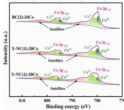
Fig 6 XPS spectra of Co 2p in BC(2)-20Co, Y-NC(1)-20Co and Y-NC(2)-20Co
